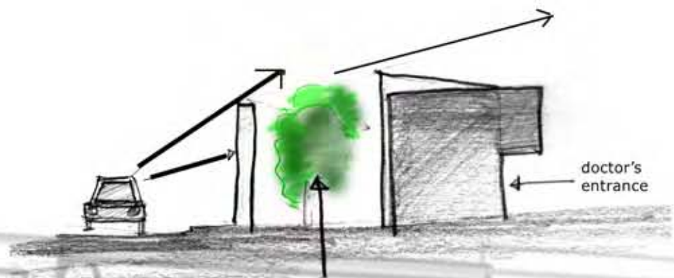
The shaded inner courtyard partially shields the clinic from noise from the road creating a welcoming and less inhibiting entrance.
